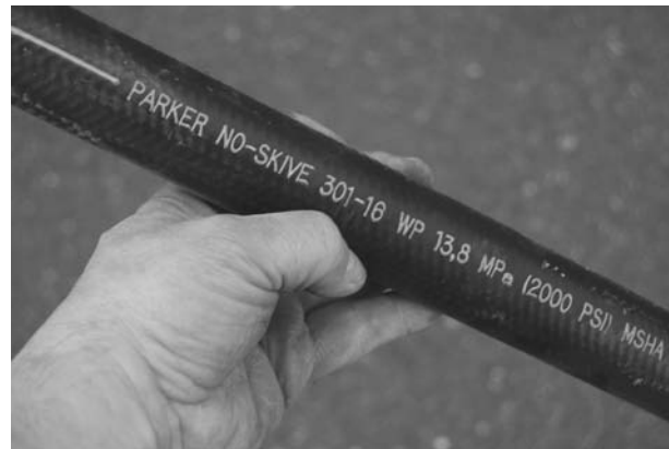
Figure 6-9 Every hydraulic hose is marked with information from the manufacturer. This information usually includes the name of the manufacturer, any unique features of the hose, industry standards to which the hose is built, and burst pressures. This hose is a no-skive hose. This means that when the hose was built, there was no modification, shaving, or cutting of the end of the hose to install the fittings. The numbers 301-16 WP indicate the manufacturer series, size, and type. Crucial for the technician to double-check is the rated burst pressures of the hose. This hose has a burst pressure of 13.8 megapascals. A megapascal is roughly equivalent to 150 psi. Notice that this hose is also marked in psi. The MSHA indicates that the hose has been designed and built in accordance with standards established by the Mine Safety and Health Administration.
