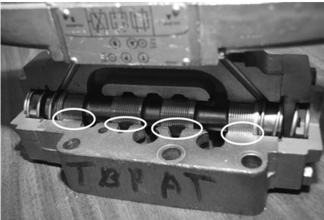
Figure 2-37 The ovals on this photo show points where the valve must seal against pressures as high as several thousand pounds per square inch. These high pressures are sealed by closely toleranced machined surfaces between the spool and the valve body. If the spool valves become damaged or even slightly abraded, they can fail to seal properly, causing erratic operation or no operation of the fluid power system.
