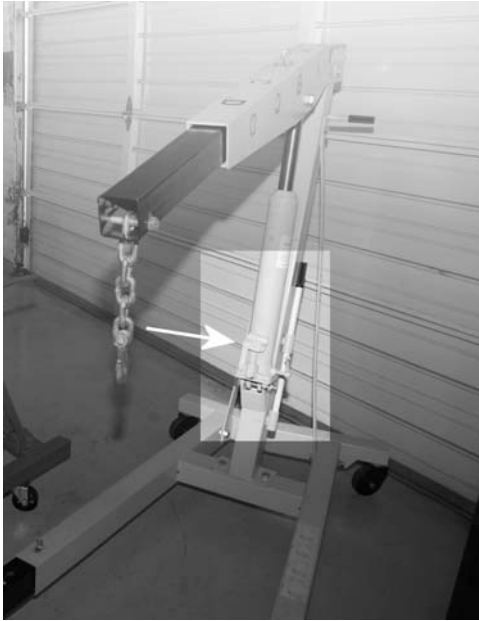
Figure 2-22 All hydraulic pumps must have a power source. In mobile equipment, the most common sources are electric motors, gasoline engines, and diesel engines. This engine crane is an example of a very simple hydraulic system. The manually operated pump is shown in the highlighted area.
