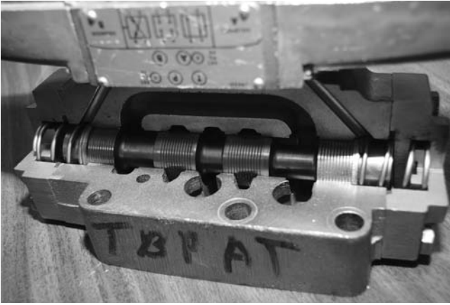
Figure 2-36 This is a cutaway of a directional control valve. The spool that runs through the center of the valve is moved back and forth to direct the flow of hydraulic oil through the system. The closely machined spool seals against very high pressures and yet must slide freely into its various positions.
