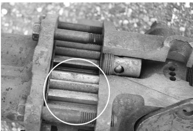
Figure 2-28 Contamination can lead to severe damage in all components of a fluid power system. Since the pump receives the hydraulic oil directly from the reservoir, it may be the most vulnerable to this damage. This shows the result of hard particle damage to the pump gears. The wear on the gear limits the flow and pressure capability of the pump. (Note: this pump has been cut open to reveal the damaged gears in place for instructional purposes.)
