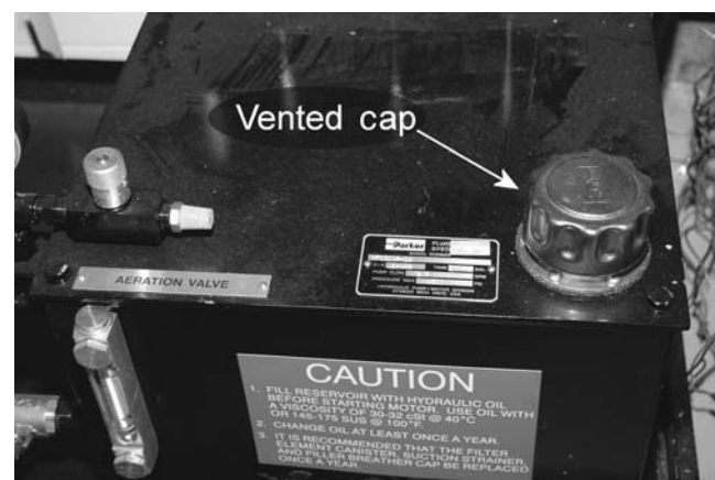
Figure 2-10 Although many reservoirs will have separate vents, many have the vent in the cap. Since this is where air enters the reservoir to push the fluid toward the pump, this vent must be filtered. In this system, the vent is in the reservoir fill cap. These caps should be routinely inspected to ensure that the filtration material is in place and is not damaged or contaminated.
