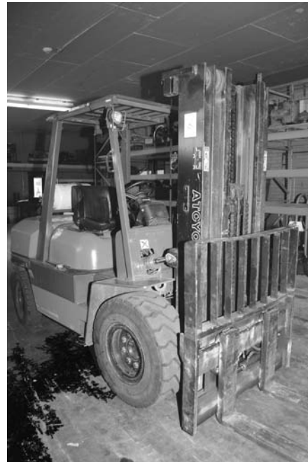
Figure 2-9 A damaged reservoir can leak hydraulic fluid. In addition to creating a mess, hydraulic oil may not be compatible with materials used in other systems on the vehicle. Wheels, tires, drive belts, wiring insulation, brake linings, and even battery cases can be damaged by some hydraulic fluids.
