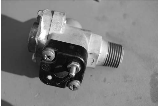
Figure 10-6 Hydraulically operated safety switches should also be inspected for proper function. Although most fluid power systems have pressure relief valves and other safety mechanisms to ensure that the system is not overpressurized, thus leading to a catastrophic failure of the hoses and other components, electrical safety switches to shut off the pump or change the position of the directional control valve are also essential for safety. At least inspect them to make sure there is no evidence of physical damage or leakage. If the design of the system permits, it would also be a good idea to pressurize the portion of the system being monitored by the pressure switch to the point where the switch should cut off. This will verify that the safety function operates properly.
