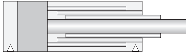
Figure 4-12 A telescoping cylinder.
