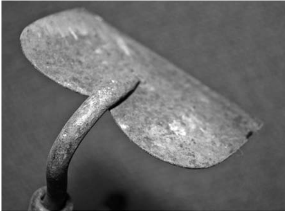
Figure 5-9 Rust and corrosion form when bare metal is exposed to the oxygen in the atmosphere. The presence of moisture can accelerate the process. Good hydraulic oil will have additives that will slow or inhibit the formation of rust and corrosion.
