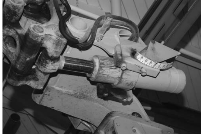
Figure 6-1 The proper installation of the appropriate type of hose can result in long-lasting, problem-free operation for the equipment. When hoses are installed, they must be of sufficient length to allow for the free articulation of the equipment. The hoses should also be bracketed to prevent them from rubbing on components as the equipment moves. Eventually normal equipment articulation will result in deterioration of the hose. When this occurs, the hose should be replaced immediately since it poses a threat to the operation of the equipment and thus is a safety hazard.
