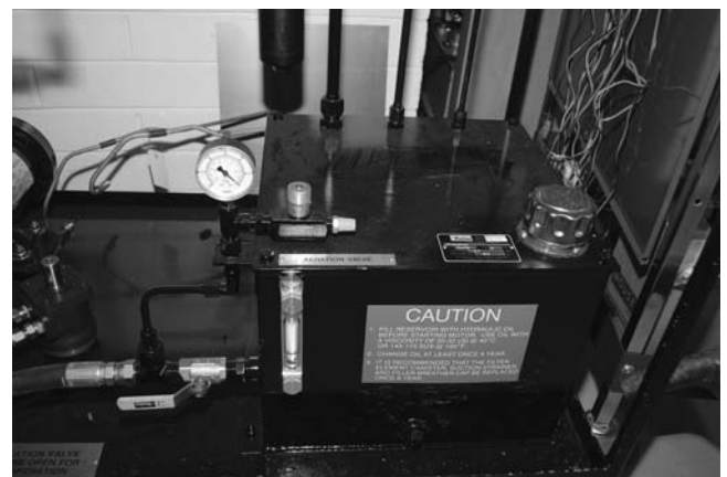
Figure 2-3 Hydraulic reservoirs come in an almost infinite number of shapes, sizes, and materials. A common material used in mobile hydraulic systems is steel. It is relatively lightweight, very strong, and does a good job of transferring the heat of the fluid returning from the working system to the surrounding air. Like many fluid power systems found on mobile equipment, this reservoir features a sight glass for easy observation of the fluid level.
