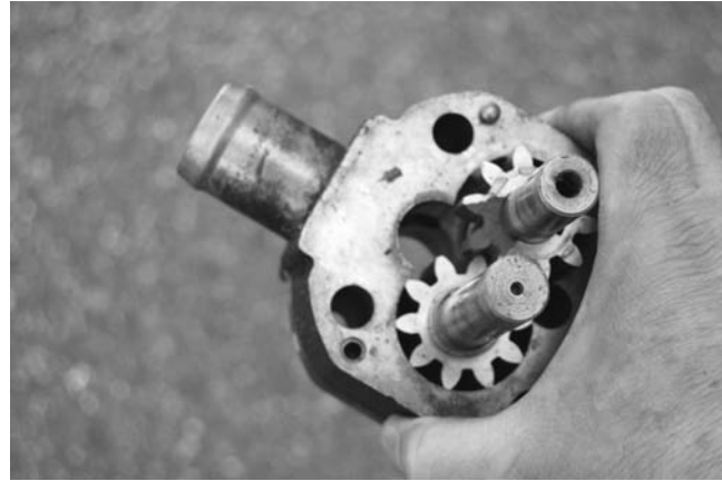
Figure 2-47 This hydraulic motor is a simple gear motor. Notice that the return line slides onto a simple tube fitting designed to accept a rubber hose and a clamp. This indicates it is a unidirectional motor. If it were bidirectional, then both hoses would have to be attached to the motor with high-pressure fittings.
