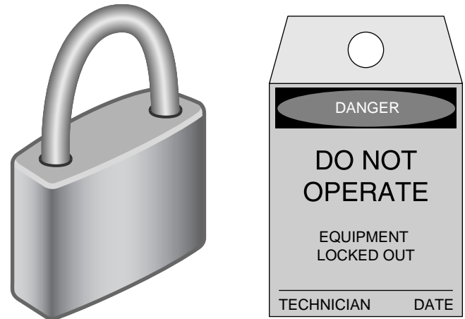
Figure 1-3 Locking out the operating controls for fluid power systems ensures that the machinery cannot be operated while maintenance or repairs are being performed. Tagging the lock and/or operating controls provides anyone attempting to operate the equipment with a warning and information about who to contact.
