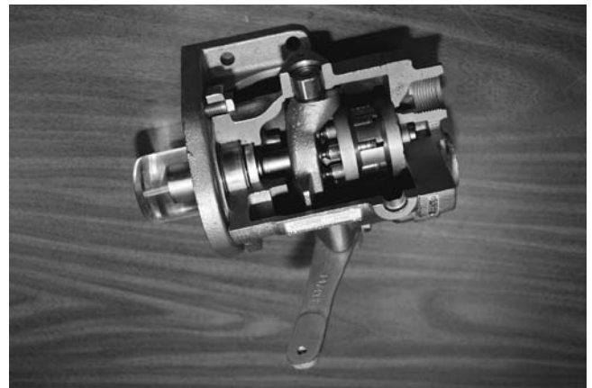
Figure 2-21 The variable displacement piston pump uses an array of pistons mounted in a set of rotating cylinders. The end of these pistons ride on a device called a swash plate. Even when the speed of the pump is held steady the volumetric flow can be altered by changing the angle on the swash plate. The swash plate angle can be altered in many ways. In the case of this pump, the angle is varied by means of the lever at the top of the photo.
