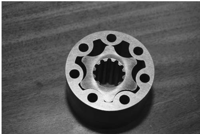
Figure 2-19 This is a variation of the gear pump. Called an internal gear pump, they offer quieter operation. As the inner and outer gear mesh, the hydraulic oil is squeezed and accelerated forward through the system.
