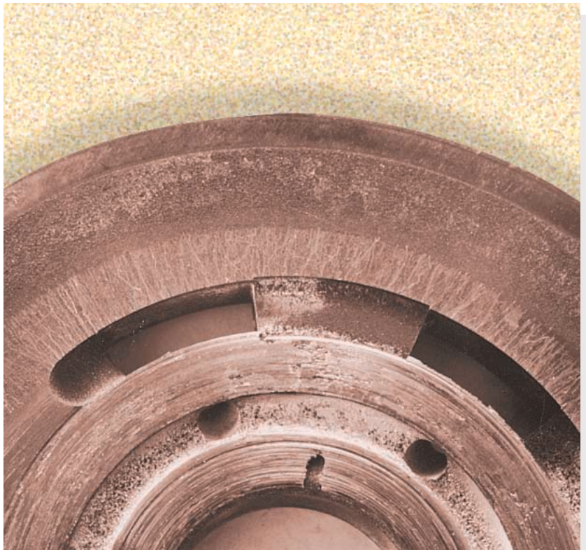
Typical results of pump wear due to particulate and water contamination
