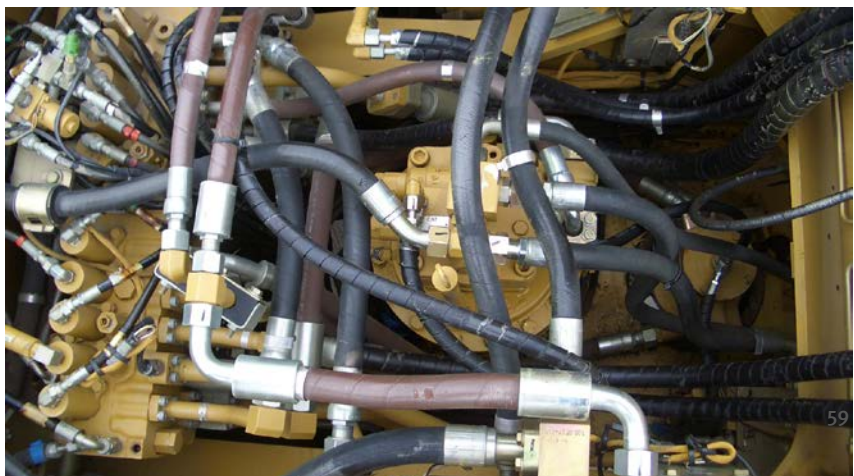
Fig. 32 Hose assemblies on a mobile hydraulic system
