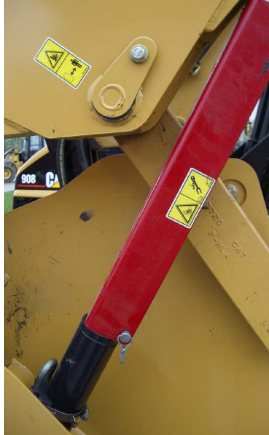
Fig. 41 Supporting device in place on an earth-moving machine
