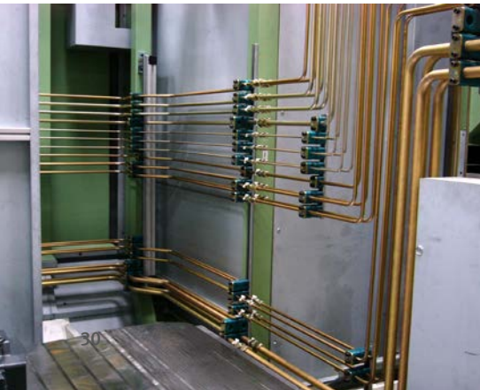
Fig. 10 Proper attachment of pipelines with pipe supports
