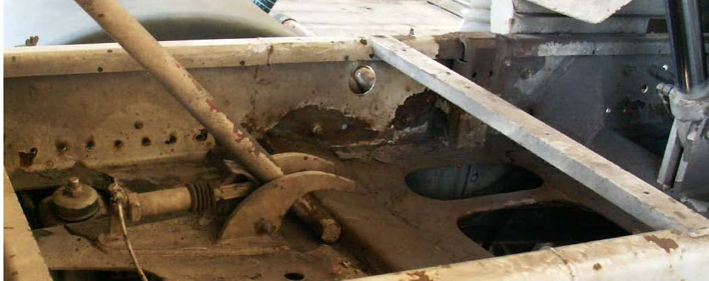
Fig. 37 Safety support on an hydraulically elevated vehicle superstructure
