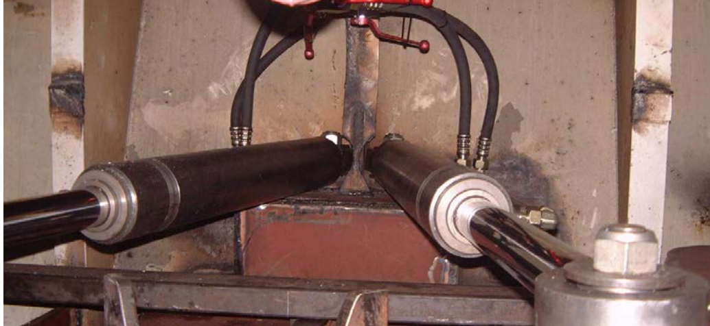
Fig. 43 Risks of pinching on a rudder system
