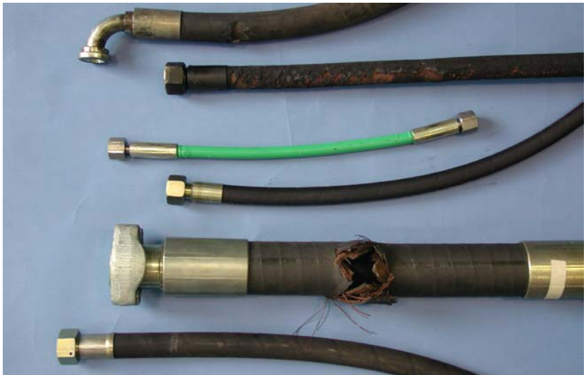
Fig. 16 Examples of failed hydraulic hose assemblies
