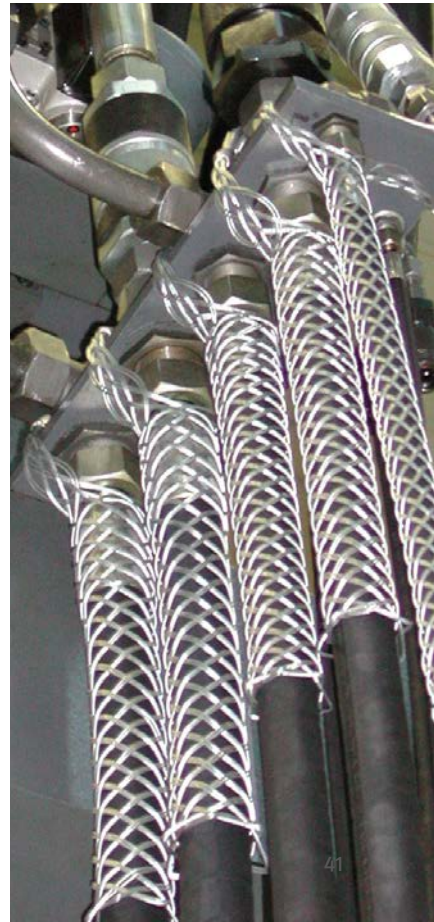
Fig. 17 Stripping protection on hose assemblies
