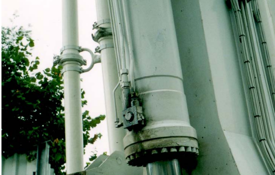
Fig. 18 Hydraulic cylinder with pilot-operated check valve
