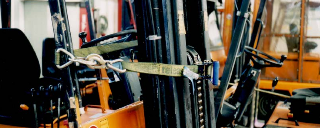
Fig. 36 Lashed lifting frame when working on tilting cylinders
