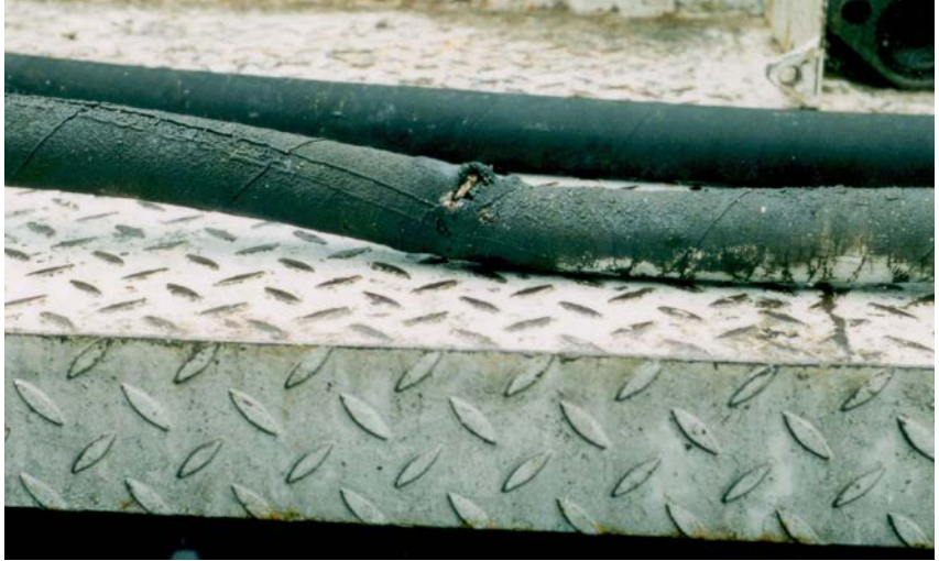
Fig. 2 Bursted hydraulic hose assembly
