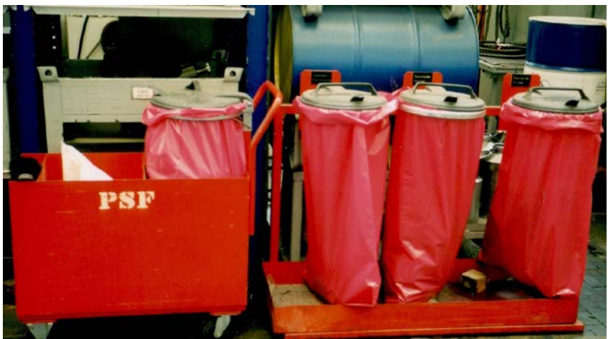
Fig. 7 Trolley for transporting oil binders
