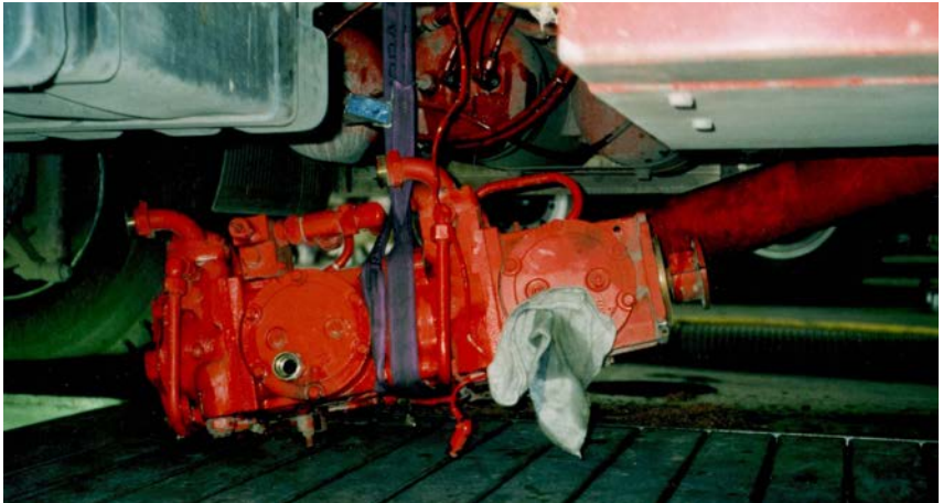
Fig. 39 Vehicle main pump on a load lifting device
