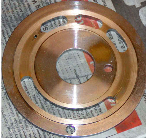
Figure 1. Scoring damage to valve plate
