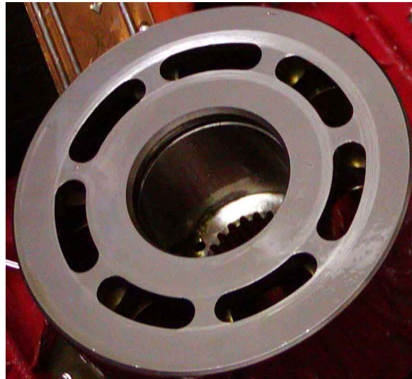
Figure 3. Scoring damage to cylinder barrel
