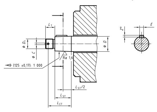
Dimension Z is normal to the key and at the large end of the taper.
