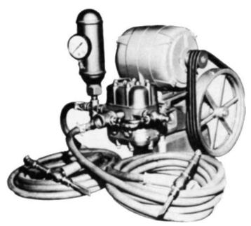
**Figure 6-1** Double-acting, high-pressure, horizontal duplex reciprocating piston pump. This pump has two cylinders and is capable of capacities ranging from 5 to 9 gallons per minute at working pressures up to 350 psi.
