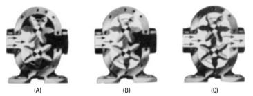
**Figure 4-2** Movement of a liquid through a gear-type hydraulic pump: (A) liquid entering the pump; (B) liquid being carried between the teeth of the gears; and (C) liquid being forced into the discharge line.
