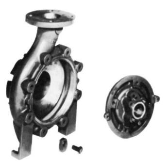
**Figure 3-18** An offset-volute design of casing (left) and cover (right). The casing is designed for top centerline discharge, self-venting, and back pullout. (*Courtesy Buffalo Forge Company*)
