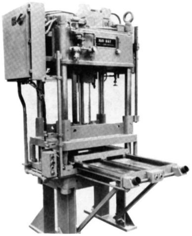
Figure 9-3 A 28-ton hydraulic trim press.
