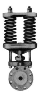
**Figure 7-15** A shock-absorbing alleviator. Hydraulic system shocks are absorbed safely and smoothly by means of a packed spring-loaded plunger that rises to relieve sudden pressure surges.
