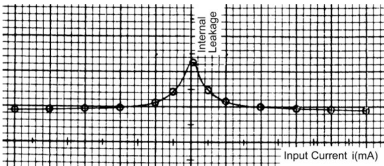
FIGURE 9.16 Typical leakage characteristics of a servovalve. (Courtesy of Moog Inc.)
