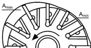
FIGURE 4.31 Location of maximum and minimum chamber volume.
