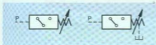
Fig. 38: Piston pressure switch, type HED1 (left) with and (right) without drain case port
