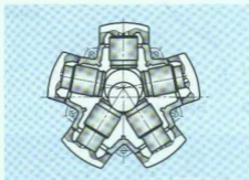
Fig. 4: Radial piston motor with internal eccentric
