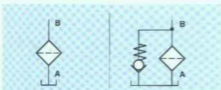
Fig. 16: Symbol for suction line filter; (left) without and (right) with by-pass valve
